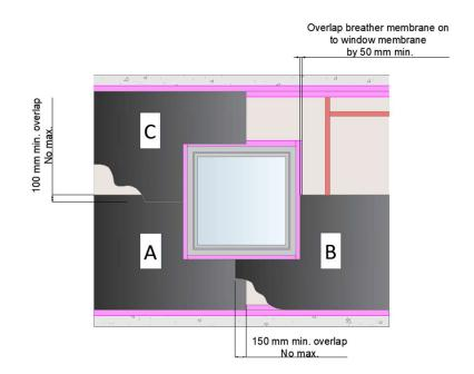
Horizontal overlaps are sealed with the self-adhesive bonding strips. Vertical overlaps are sealed with the correct illbruck tape, applied bubble and wrinkle free and all bonds are consolidated with a seam roller.
