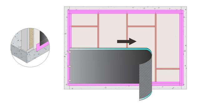
Unfurl the membrane horizontally and press the self adhesive strip on to the substrate ensuring that the membrane is applied smoothly and free from wrinkles and bubbles. Sections of masking tape can be applied on adhesive free edges if required to temporarily secure the membrane in position.
