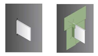
All incisions around any penetration are fully sealed with the correct illbruck tape.
