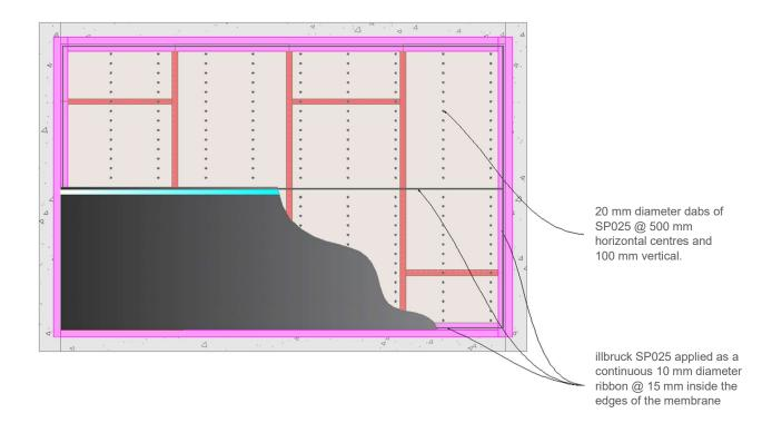
For low to medium wind loads a 10 mm diameter bead of SP025 adhesive should be applied around the entire perimeter of the membrane. For higher wind loads, the bond can be further enhanced by applying 20 mm diameter dabs of SP025 Fire Membrane Adhesive at 500 mm horizontal and 100 mm vertical centres.
