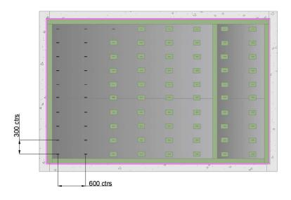
For other sheathing boards and substrates where staples are not suitable or for a more robust fixing method, stainless steel screws are installed through the sheathing board into the SFS at 500 mm centres vertically and to align with every stud.
