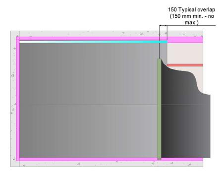
Once the joints have been formed and the membrane is temporarily secured, apply the correct illbruck tape to seal the overlap. The tape should be wrinkle and bubble free, and the bond consolidated with a seam roller.
