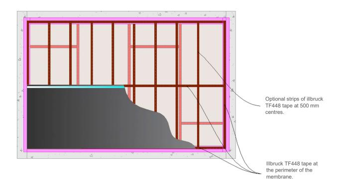
For low to medium wind loads the double sided tape should be applied around the entire perimeter of the membrane. For higher wind loads, the bond can be further enhanced by installing vertical strips of TF448 High Performance Bonding Tape at 500 mm centres.
